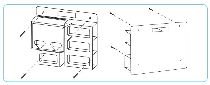
Wall Mount: Securely mount unit to a wall via keyholes and screw holes in back with screws approved and supplied by building maintenance. All four
